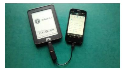
8. If the kobo is off, it will boot into XCSoar so exit the programme and connect to Nickel (bottom left button). Select 'connect' when the option to 'computer detected/connect to a computer' comes up.
